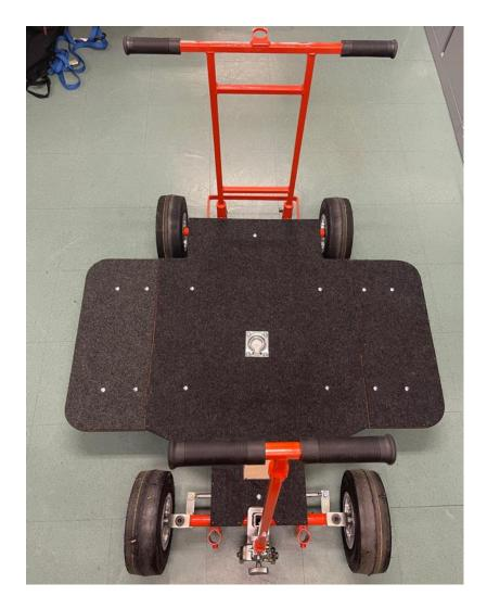
Press the blue button on the Tow Receiver Pin to remove it. Slot the Tow Bar into the Tow Receiver, insert the Pin and tighten Thumb Nut. You may now pull the dolly and steer it.
