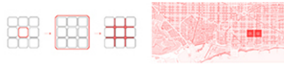
Fig. 1 1859 Example block, new Superblock three-by-block area with periphery streets, and Superilla interior pedestrianized streets of limited vehicular traffic
