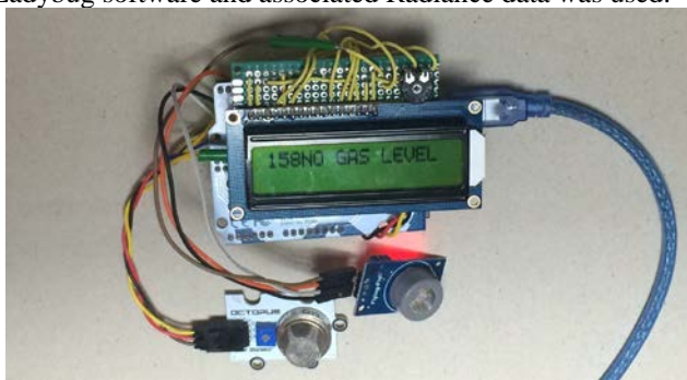
Fig. 4 Arduino microprocessor based sensor platform with gas sensors (Image by BettyLou Poston)
