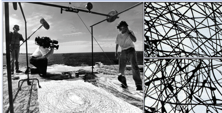
Left: The author demonstrates a kicked pendulum (see p41) for ABC Television. Right: Examples of non-chaotic (top) and chaotic (bottom) patterns produced using the pendulum.
