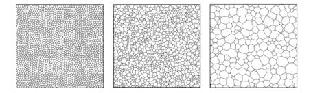
Fig. 4. Simulations by Drenckhan of the evolution of a foam as a function of time.
