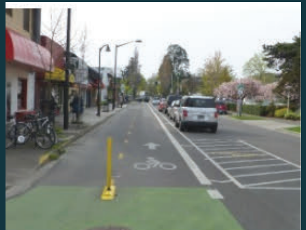
Two-way cycle tracks provide a comfortable experience for people riding their bicycle
