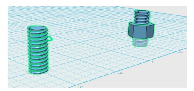
With the suggestion from the tutorial, I rotated the bolt 180 degrees so that the flat head would be the base to ensure proper printing.
