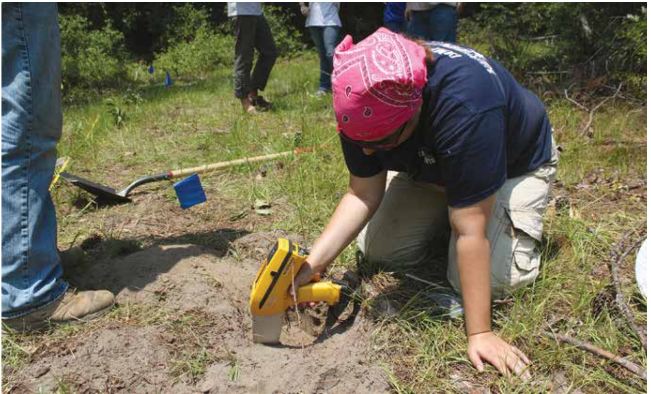
Amanda Morrow uses an x-ray fluorescence machine to measure the corrosion of in situ artifacts. This information helps the researchers to determine how best to conserve the corroded items.
