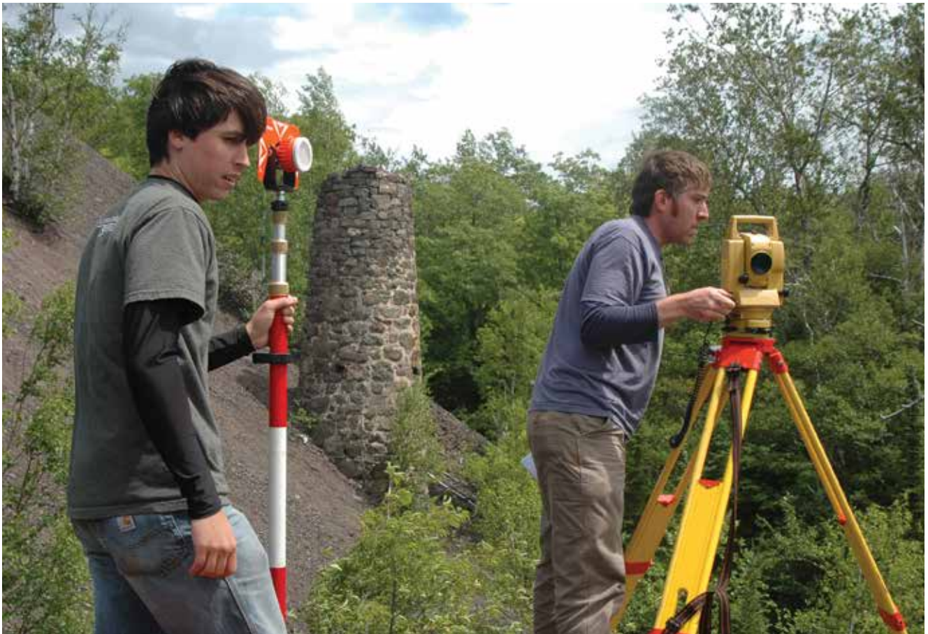
James Dau and Sean Gohman collect digital survey data while mapping the site in 2010. Mine waste has buried part of the 1860s' chimneystack in the background.
