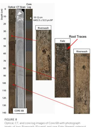
insets of two Riverwash (Fluvent) and one Fiale (Xerept) paleosol. White star on core log shows location of radiocarbon sample and depth and age are noted. Red arrow shows location of paleosol. Distinct root traces are noted in the Fiale.
