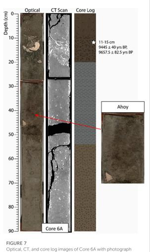
Optical, CT, and core log images of Core 6A with photograph inset of Ahoy (Xeroll) paleosols identified in core. White star on core log shows location of radiocarbon sample and depth and age are noted. Red arrow shows location of paleosol.
