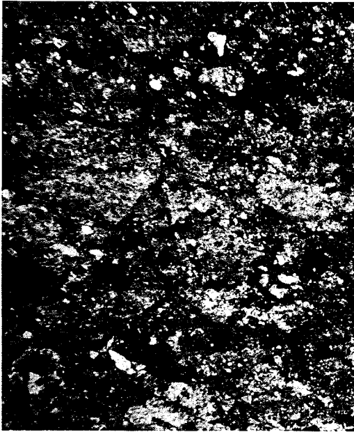
Fig. 15. Vomosepic porphyroskelic plasmic fabric with fine granular peds defined by ferrans, from B_{3ird} horizon to type Long Reef clay palaeosol (UNER35272b, x25).
