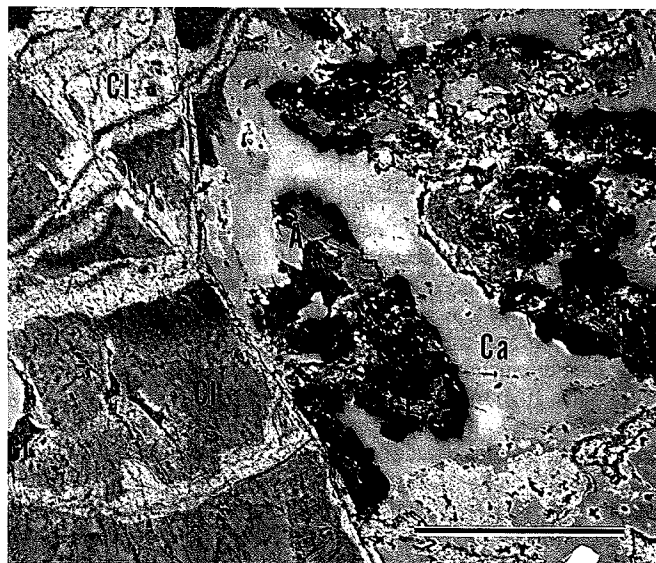
FIG. 7.—Back-scattered electron micrograph of hornblende (A) weathered to carbonate (Ca) and three kinds of chlorite (Cl), light (Fe-rich), medium, and dark (Mg-rich), from the type Staca clay (R337). Scale bar 50 \mu\text{m} .
