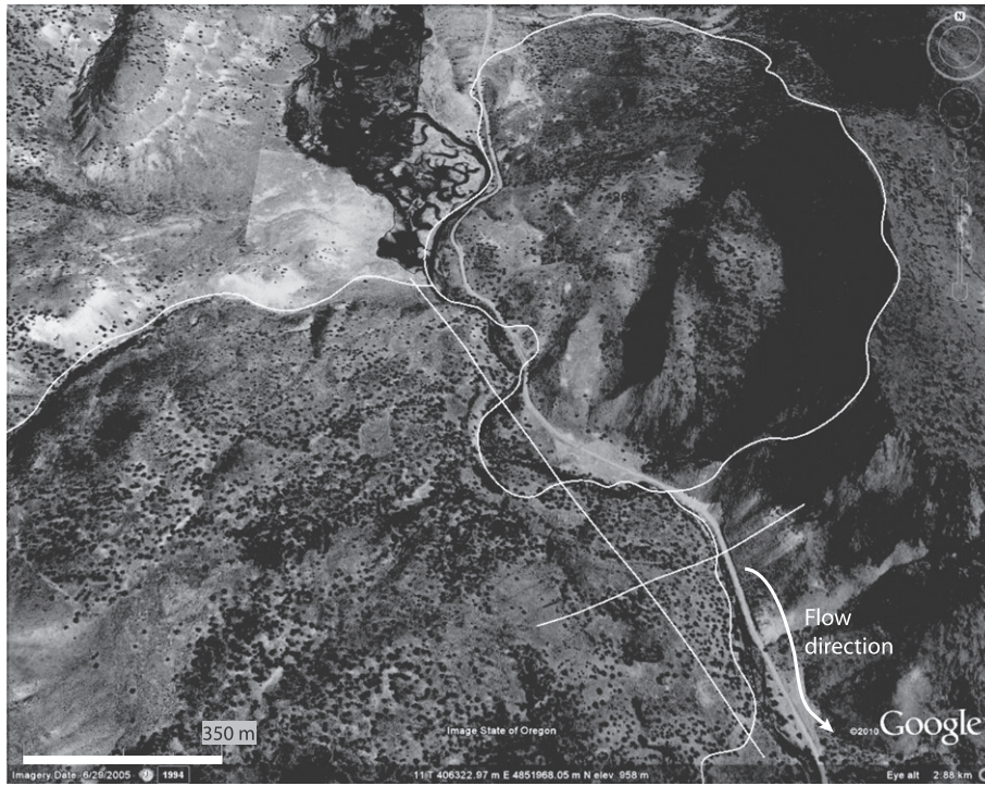
Fig. 9. Oblique Google Earth image of Chukar Park landslide dam site. North Fork Malheur River flows from top to bottom of image. A pair of landslide complexes, outlined in white, flank the river on both sides. Based on field observations, the landslide dam crest is believed to be along the short, valley-perpendicular line, and the breach zone is spanned by the long, valley-parallel line.
