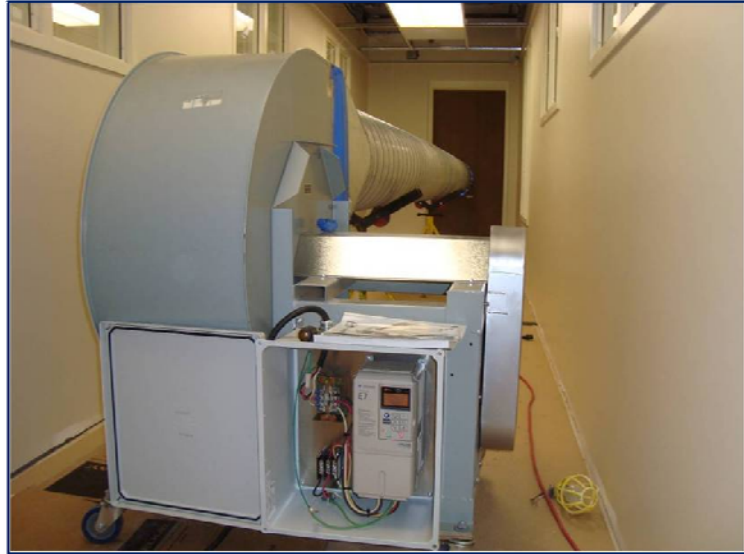
THE STAGING EQUIPMENT FOR A BLOWER-DOOR TEST. - IMAGE COURTESY OF USACE, KANSAS CITY DISTRICT.
