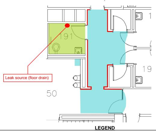
\*NOTE: LEAK SOURCE WATER IS CATEGORY 3 (BLACK WATER). PLEASE DISINFECT ALL IMPACTED SURFACES FOLLOWING REPAIRS AND BULK CLEAN UP.
