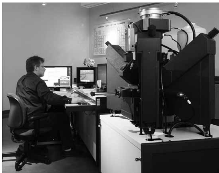
John Donovan using a Cameca SX50 Electron Microprobe Analyzer in the MicroAnalytical Facility in the Lokey Laboratories.
