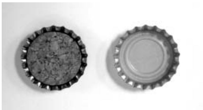
A "crowning" achievement. Left: old-style bottle cap sealed with a cork disc. Right: a bottle crown with a modern synthetic organic seal.
