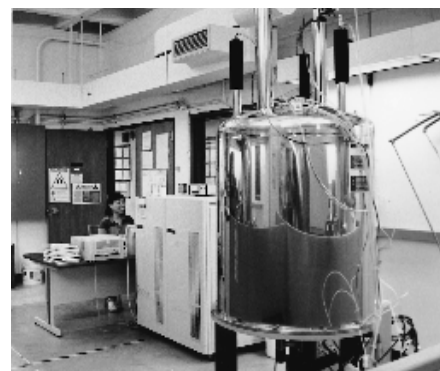
Myungok Yoon works in the third-floor instrumentation facility with Varian INOVA-300 NMR spectrometer.
