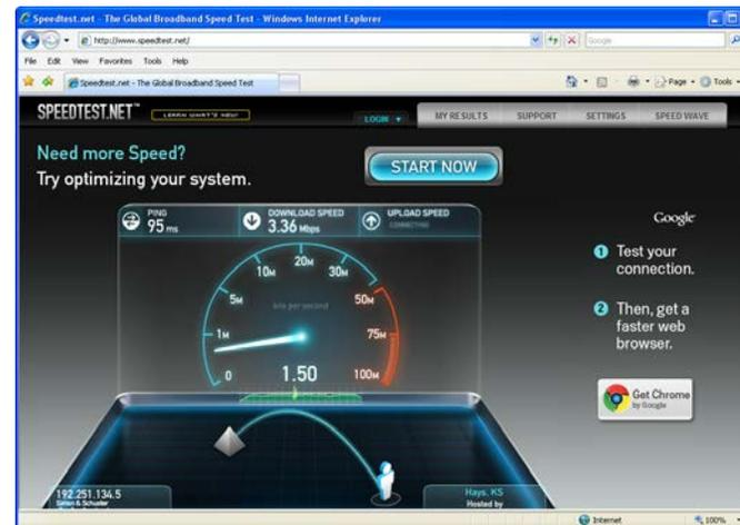
6. At the conclusion of the speed test, your results are displayed. The download and upload speeds are provided in Mbps (Megabits per second).
