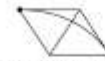
DRAW CURVE TANGENT TO BOTH EDGES LOCATE CURVATURE POINT ON DIAGONAL LINE
